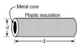
Plastic insulation surrounds a wire having diameter d and length l as shown above. A decrease in the resistance of the wire would be produced by an increase in the
